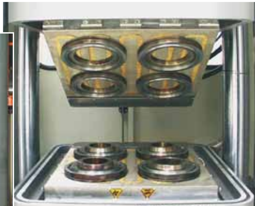
M-TECS 240-G on a vertical press – various shapes on a machine bed without loss of space due to clamping claws
